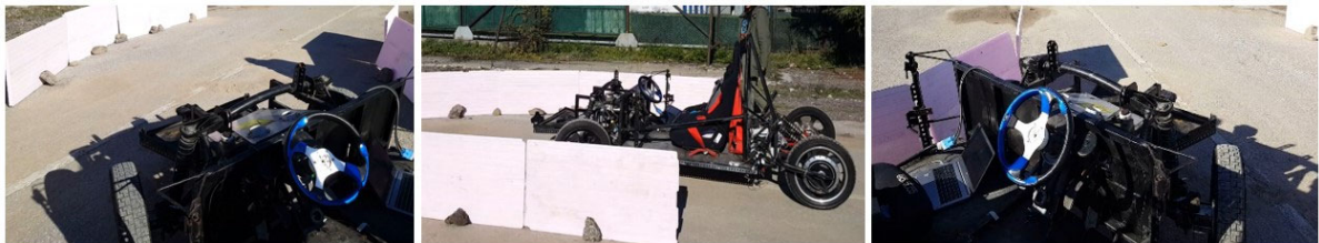
Fig. 7. Real time control command testing towards safety level verification with LiDAR data. (a) right turn. (b) moving straight. (c) left turn.
