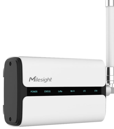
Şekil 5: Milesight IoT LoRaWAN Gateway UG65
